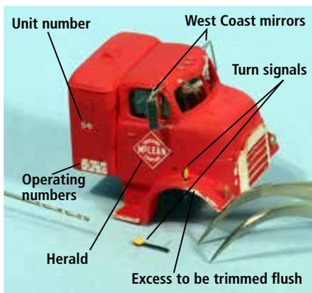
McLean was an early adopter of electric turn signals. Mounted at the top and outermost point of each tractor fender, these signals could be seen from the front and rear of the tractor.
