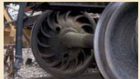
**RIBBED-BACK WHEEL.** Heat-dissipating ribs on the back of the wheel were a characteristic of many "chilled" cast-iron wheels.
