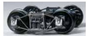
Kadee's HO scale archbar truck models an older style of truck.
