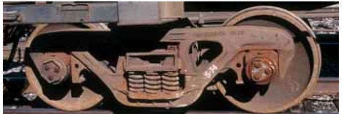
**Fig. 14 100-TON RIDE CONTROL TRUCK.** The 100-ton version of the ASF Ride Control truck has three visible springs. Note the differing styles of bearing end caps on each axle.
