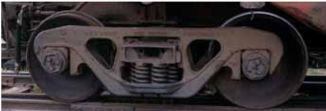
**Fig. 13 ROLLER-BEARING TRUCK.** This 70-ton ASF Ride Control truck shows the roller-bearing end caps. The roller bearing assemblies take the place of the journal boxes.
