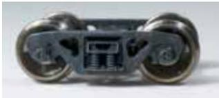
This Kato HO Barber S-2 truck features roller-bearing end caps that actually rotate.
