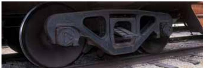
**Fig. 16 BARBER-BETTENDORF CABOOSE TRUCK.** The most popular modern-era caboose truck was the roller-bearing-equipped version of the venerable Barber-Bettendorf truck.
